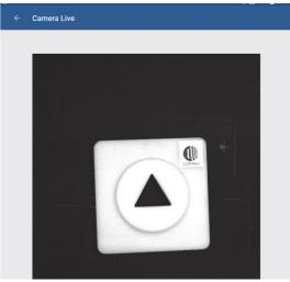
This environment allows the user adjusting the camera physical parameters (focus and diaphragm), by manually acting on it, before executing the <u>Configuration</u> procedure.
