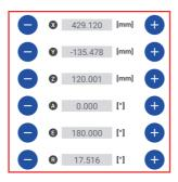
These are the cartesian coordinates of the robot current position (X, Y, Z, Euler angles).
