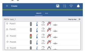
Reverse - this command copies the existing points in reverse sequence, until the second one. This allows to move along the path backward, and restart the cycle from the beginning.
