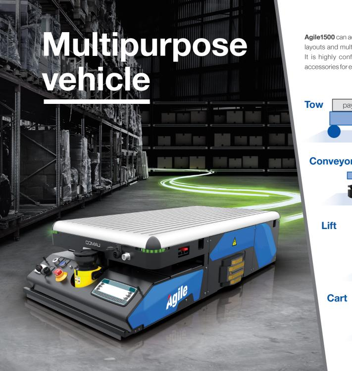
Agile1500 can adapt to accommodate diverse manufacturing needs, factory layouts and multipurpose application possibilities.
